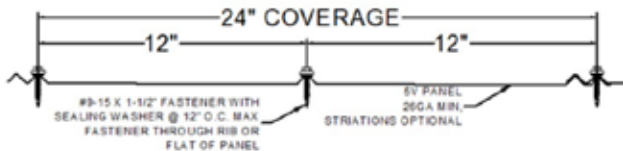
PATTERN A6 12"-12" FASTENER PATTERN FASTENER ROW SPACING: 6" OC
