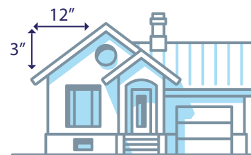
Determining Roof Pitch/Slope
