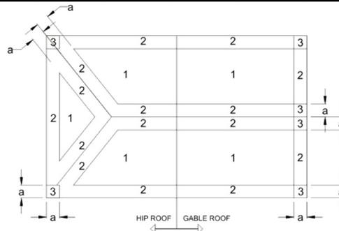
a: 10% OF LEAST HORIZONTAL DIMENSION OR 0.4ft, WHICHEVER IS SMALLER, BUT NOT LESS THAN EITHER 4% OF LEAST HORIZONTAL DIMENSION OR 3FT (0.9M), OR AS DETERMINED BY REGION OR OTHER APPLICABLE CODE.
