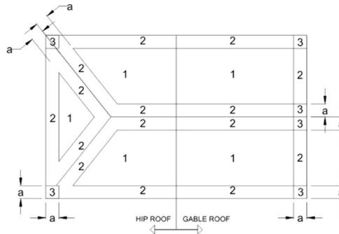
※ 10% OF LEAST HORIZONTAL DIMENSION OR 0.4', WHICHEVER IS SMALLER, BUT NOT LESS THAN EITHER 4% OF LEAST HORIZONTAL DIMENSION OR 3FT (0.9M), OR AS DETERMINED BY DESIGN OR OTHER APPLICABLE CODE.
