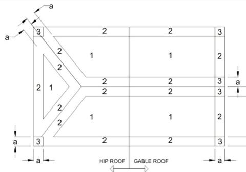
• 10% OF LEAST HORIZONTAL DIMENSION OR 0.4L, WHICHEVER IS SMALLER, BUT NOT LESS THAN EITHER 4% OF LEAST HORIZONTAL DIMENSION OR 3FT (0.9M), OR AS DETERMINED BY DESIGN OR OTHER APPLICABLE CODE.
