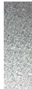
**Mill Finish** is not an architectural coating and therefore susceptible to a differential weathering. This weathering or discoloration does not affect the product performance or the finish warranty therefore is not a cause for rejection.
